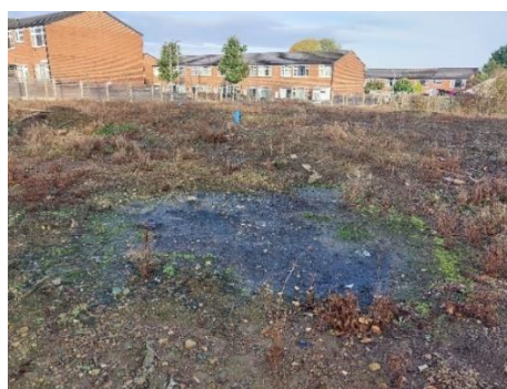
Figure A – Exposed spent oxide impacted soil at Buckle Lane, Normanton
