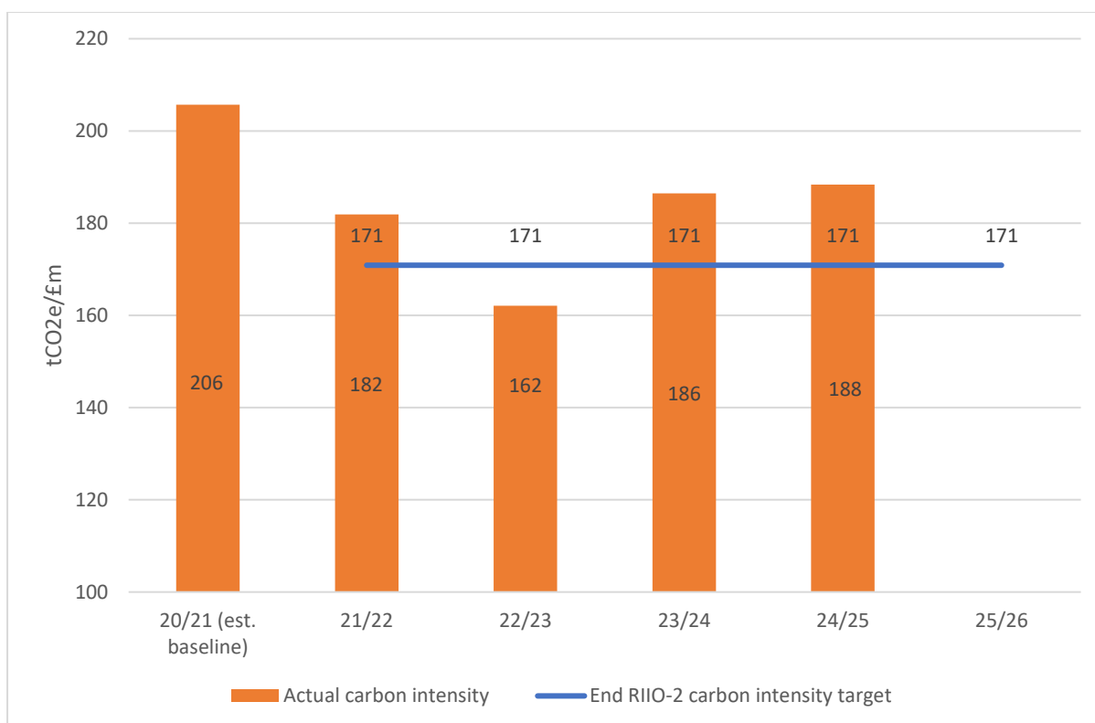
Figure 11 – Estimated embodied carbon emissions intensity for gas mains replacement, diversions and reinforcements (<7 barg), new connections and emergency repair work in 2020/21 prices
