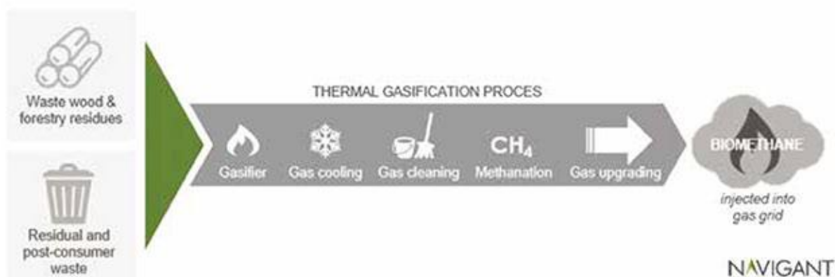
Figure 30 Schematic overview of the thermal gasification process
