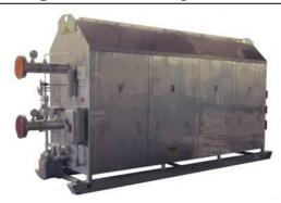
HotCat's are made up of several zones each containing 2 catalytic heaters. Each zone can be controlled independently. Bruest state in their literature that the efficiency of their system is 70%. However, this figure does not include electricity consumption. Before the gas supply is provided to each heater, the catalyst needs to be preheated to 232°C by an electrical preheating element. Once achieved, the electrical supply is disconnected and gas combusts to provide all of the required heat.
